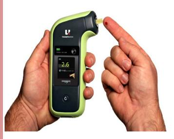
The patient or other user inserts a test strip into the meter and after the finger is pricked, touches the tiny drop to the biosensor strip
