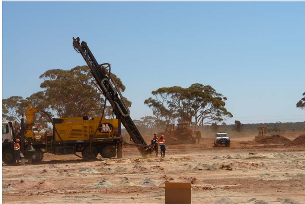
Figure 3: Grade control drilling in progress at Costello Open Pit.
