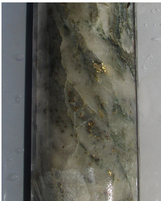
Drill core showing visible gold located 150 metres south of the dolerite dyke 30 metres below 23 level.
