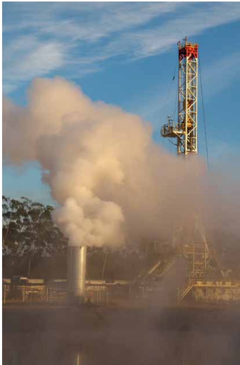
Salamander-1 clean-up flow test, May 2010.
