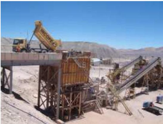
A 30 ton truck discharging ore for crushing.
