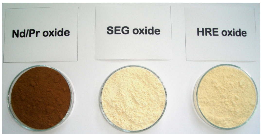
Rare Earth Oxide samples for customer evaluation produced from Nolans Bore mineral concentrate.
