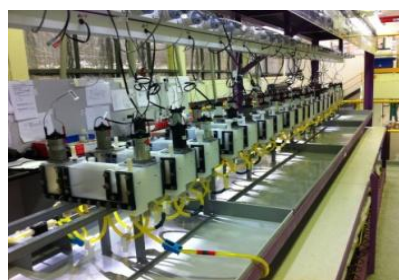
Solvent extraction circuit for REO production ANSTO
