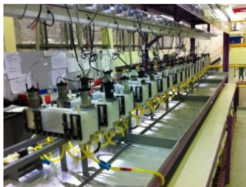
Solvent extraction circuit for REO production – ANSTO
