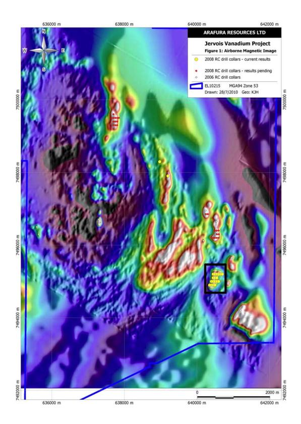
Figure 1: 2008 and 2006 RC drill hole locations, Jervois Vanadium Project, NT. The location of the Casper prospect is shown by the black box.
