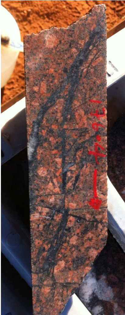
Chlorite / Biotite / Qtz fractures / stock-working in porphyry – typical grade 0.2 to 1.5g/t Au over wide widths.
